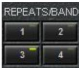
The REPEATS/BAND buttons determine how many times the scanner will scan a single band before moving on to scan the next band (if multiple bands are enabled for scanning). If only one band is enabled for scanning, the REPEATS/BAND buttons have no effect. Due to the time it takes for signals to settle when changing bands, especially when using the programmed antenna mode (discussed later in the manual), it is highly recommended that you scan a band at least twice before moving on to the next band.
