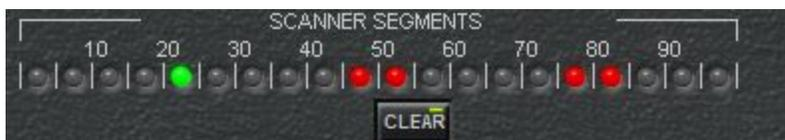
The “SCANNER SEGMENTS” LEDs are used to show which 5KHz segment of the band you are currently listening to or scanning (green LED) and which, if any, 5KHz segments of a band are currently disabled from being scanned (red LEDs). To disable a segment from being scanned (for instance, if there is a beacon or on-going QSO in that segment and you don’t want the scanner to stop on that signal), you simply click on the LED for that segment. If you have disabled multiple
